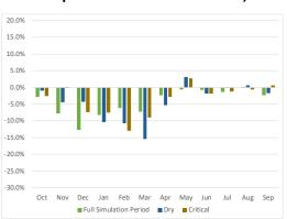
This row of charts above illustrates the increment of impact Alternative 5 Delta Tunnel conveyance and operational changes upstream would have on Delta flows at Freeport and near Hood in 2040. Decreases in flow due to Alternative 5 Delta Tunnel operations would come on top of, in addition to climate change impacts on the Delta. Y-axis ranges are identical to facilitate ready comparison.
