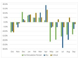
This row of charts above illustrates changes in Sacramento River flow at Freeport and near Hood to be expected just from climate change impacts on operations of SWP and CVP relying on through-Delta conveyance (that is, using existing Delta facilities). Y-axis ranges are identical to facilitate ready comparison.
